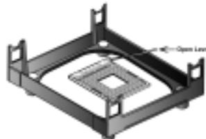
4. Locate the CPU cut edge (the corner with the pinhole noticeably missing). Align and insert the CPU correctly.
