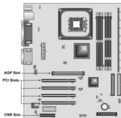
**PCI Slots** PCI slots are used to install expansion cards that have the 32-bit PCI interface.
